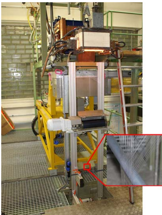
Fig. 1 Pilot plant equipment for online commingled yarn spinning of GF and PP. The insert shows the intermingling of glass filaments (perpendicular) and polypropylene filaments (from right hand side)
